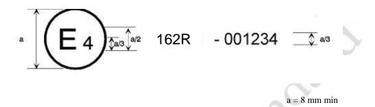
The above approval mark figure 1 affixed to a vehicle shows that the type concerned was approved in the Netherlands (E 4) pursuant to UN Regulation No. 162 under approval No. 001234. The first two digits (00) of the approval number indicate that the approval was granted in accordance with the requirements of UN Regulation No. 162 in its original form. ations
